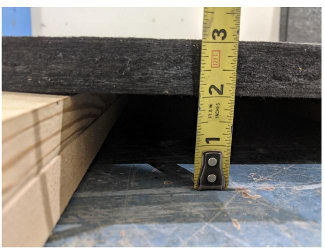
Figure 5 – Detail of specimen materials and airgap depth
