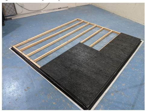
Figure 4 – Specimen partially installed over spacers
